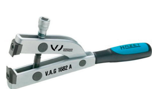
VAG1682A ASE 451 472 01 000 CLAMPING PLIERS Tool for fitting ear-type clamps used on sealing gaiters of outer drive shaft joints. The application is described in the workshop manual. Items supplied, Clamp tensioning tool, insert AF8, 3/8" drive , ASE 451 472 01 000. Produsent: Hazet-Werk
