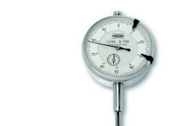
VAS 6079 ASE 469 720 00 000 DIAL INDICATOR Dial gauge designed to meet DIN 878-A standards. Measuring range: 0-10 mm. Measuring pins made from non-rusting steel. Shaft diameter: 8 mm/h6. Scale in 0.01 mm. Housing diameter: 58 mm. Supplied with plastic case. Produsent: Wenzel GmbH.
